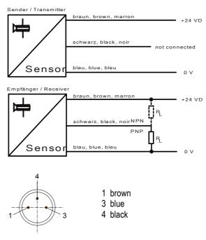
3-pin connector (view on the sensor):
