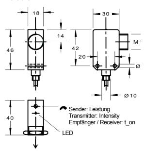
Use appropriate miniature screw driver max. size 2.5mm for adjustment of the two potentiometers.
