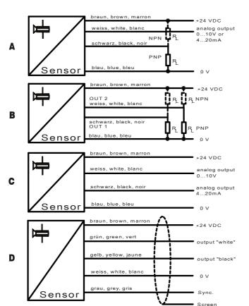
All versions with integrated cable instead of connector have cable colours according to scheme "D".
