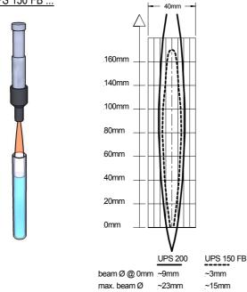
The ultrasonic sensors series UPS FB (FOCUS Beam) are equipped with a focusing device made of glass-fibre reinforced polypropylene, which makes the sound beam particularly narrow. Therefore they are suitable in the near range from 0mm up to 150mm to watch into narrow cavities. A typical application is measuring of liquid level in small tubes or containers.
