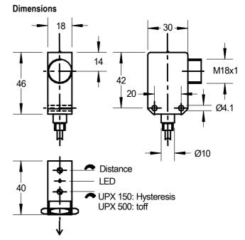
Use the miniature screw driver which is included for adjustment of the two potentiometers.
